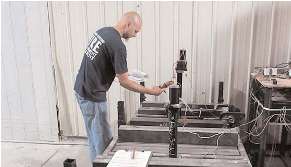
*Progressive Engineering's lab technician Chris Stutzman performs cycle testing on one of Ultra-Fab's electric tongue jacks.*
